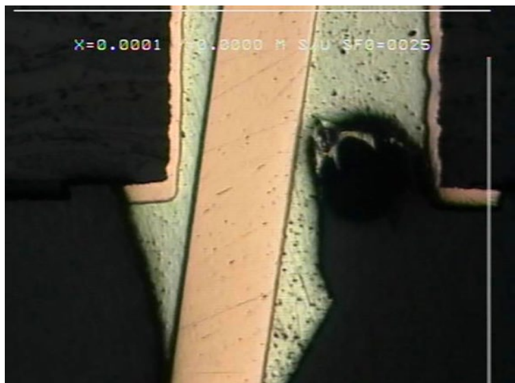
Figure 2: Poor solder flow-up and possible blowhole. (Source: Carano, Advanced Troubleshooting Course)
