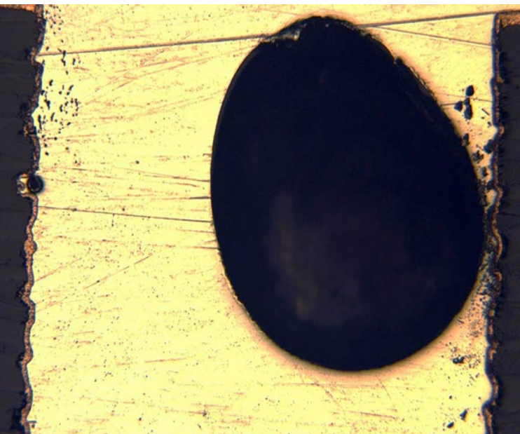
Figure 1: Blowhole or outgassing—major void in solder fillet. (Source: RBP Chemical Technology)
