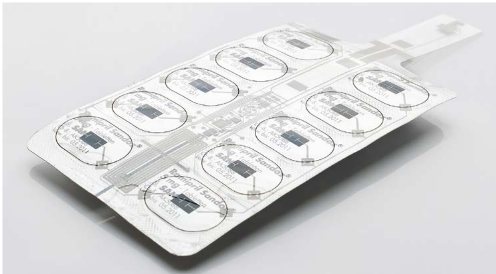
Figure 4: This hybrid smart blister pack and an additional smartphone app support patients in taking their medicine. (Source: Holst Centre)
