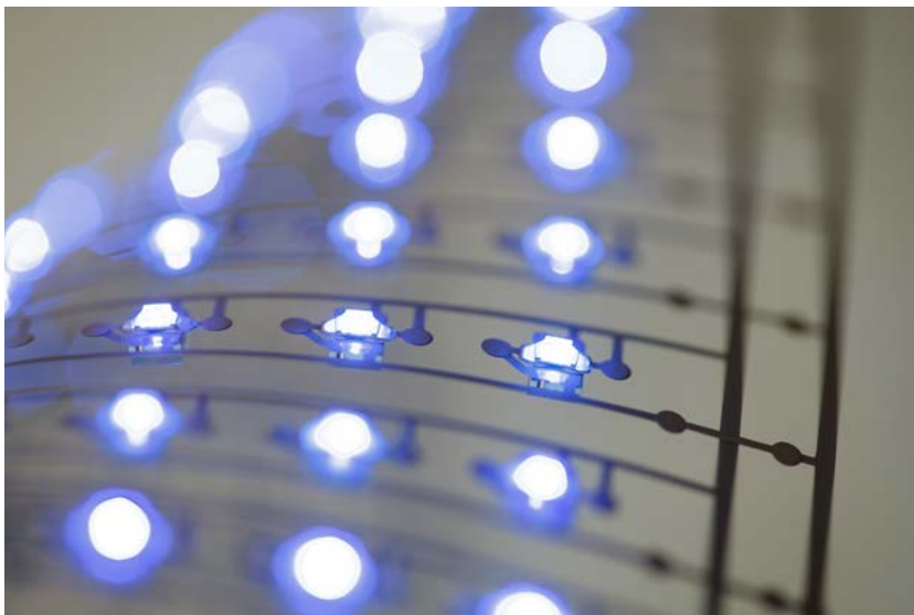
Figure 3: As seen in this lighting foil, hybrid systems bring together classical silicon and printed electronics components. (Source: Holst Centre)
