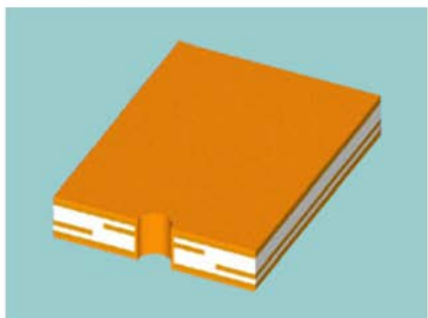
4. Holes are drilled to provide access to the multiple layers of circuits, then metallized to connect the layers electrically
